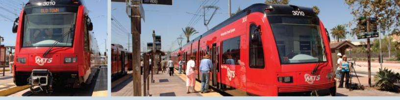
Bi-directional, six-axle, low floor articulated light rail vehicle constructed of low alloy high tensile (LAHT) steel and composite materials.
